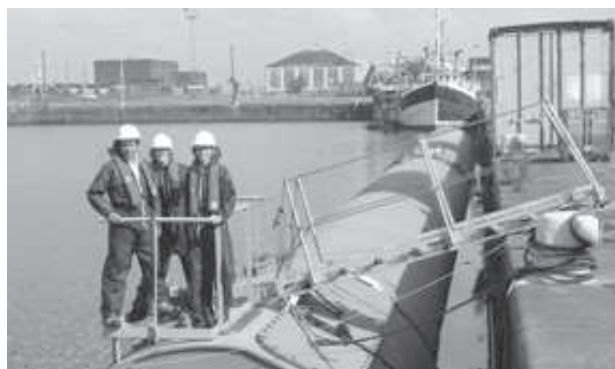
(left to right) Bob Eder, Flaxen Conway, and Kaety Hildenbrand on the 150m long Pelamis wave energy device in Edinburgh Scotland. This type of device is the first full-scale grid connected wave energy device. Three of them were recently installed off the coast of Portugal.
