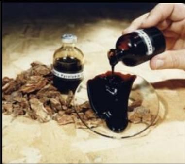
Bio-oil is perhaps the most valuable product of fast pyrolysis. It can be burned in standard boilers to produce electricity or upgraded to transportation fuel, although this is not economically viable at present.
