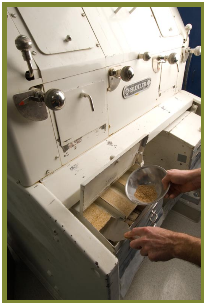
Buhler MLU-202 laboratory mill.
