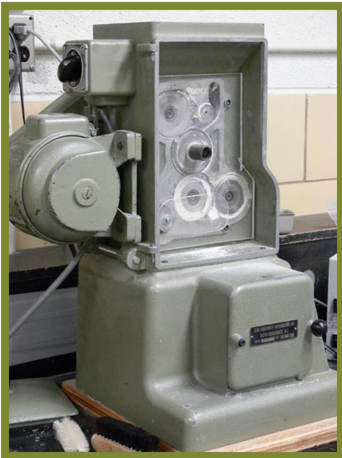
Brabender Quadramat Jr. laboratory mill.
