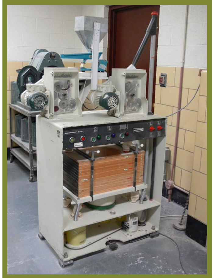
Brabender Qudramat Sr. laboratory mill.
