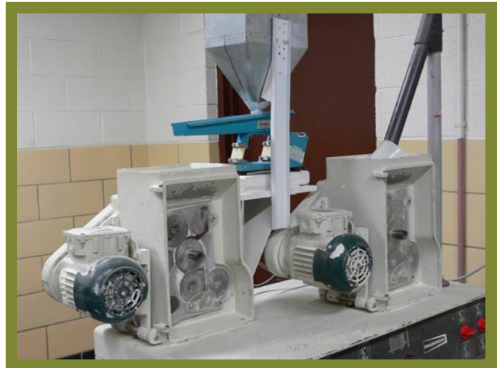
Brabender Qudramat Sr. grinding rolls.
