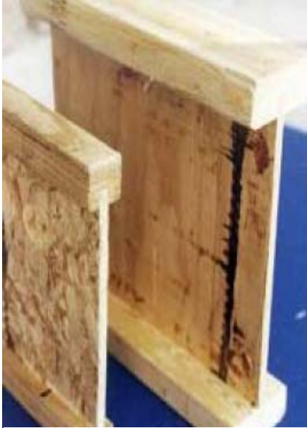
Wood I Joists—an Engineered Wood Product often used in place of solid sawn lumber to frame floor systems in homes
