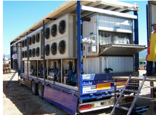
Portable hydrocoolers follow the harvest as it moves from the west coast to the mountains of the east.
