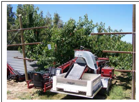
Experimental harvester used to pick fresh cherries trained to the Y-trellis system.
