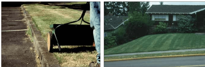
Figure 6. Drop spreaders are very accurate but must be operated properly. The lawn on the right has stripes because the operator failed to overlap each pass.
