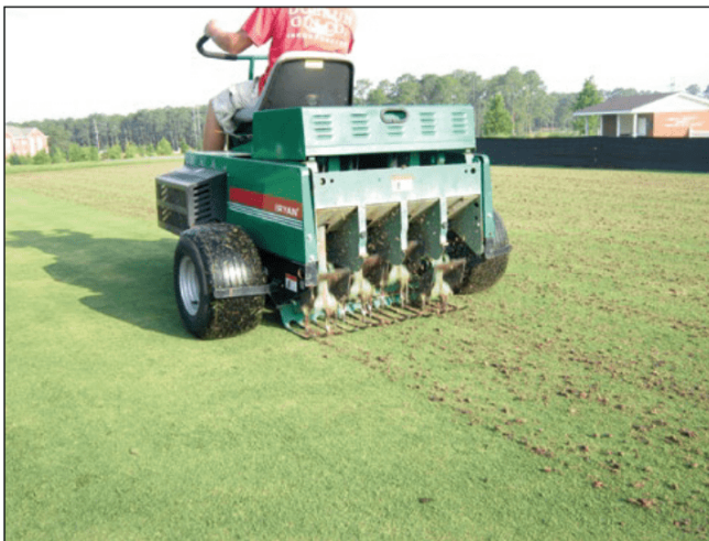
Figure 12. A core aeration unit (left) will relieve soil compaction and reduce thatch by pulling a soil core (right). these cores can be incorporated back into the turf using a rake or rotary mower.
