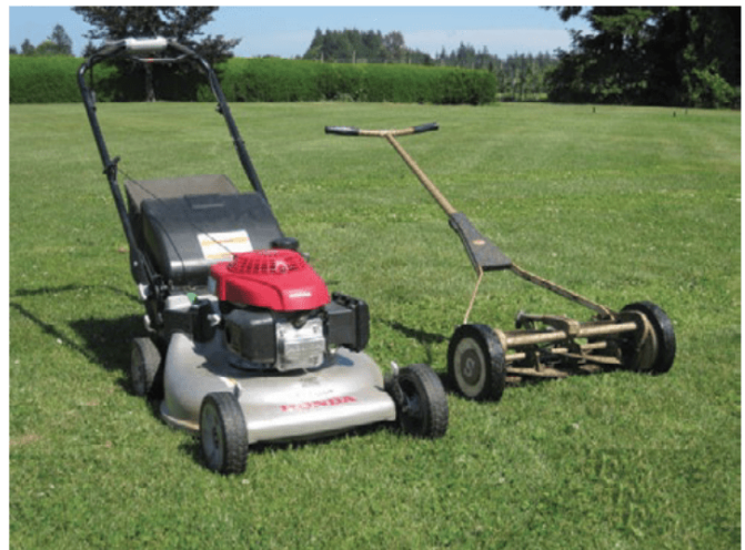
Figure 8. Rotary mower (above left), while durable, typically cannot be set to a height below 1 inch. Push reel mowers (above right) typically cannot be set higher than 2 inches
