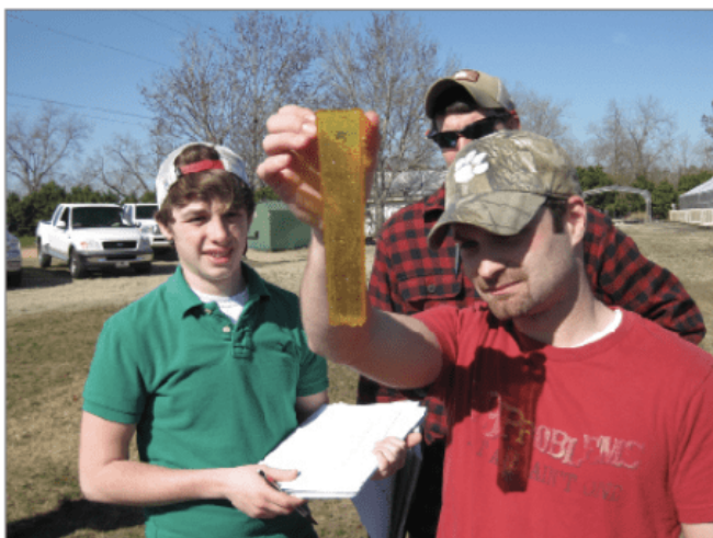
Figure 11. Use a rain gauge or catch to determine your irrigation rate in inches per hour. Irrigation events typically should not exceed 0.5 inches in a single application.
