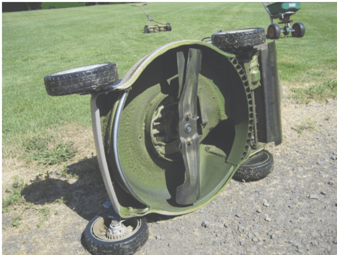
Figure 9. The double blade pattern of a mulching mower is designed to thoroughly mulch grass clippings.
