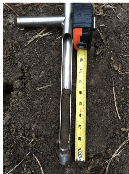
Figure 5. Measuring sampling depth
