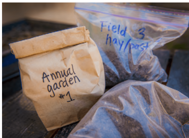
Figure 7. Take a photo of your sample bags before you mails them, for future reference. Do not use a paper bag unless the lab provides one lined with plastic.
