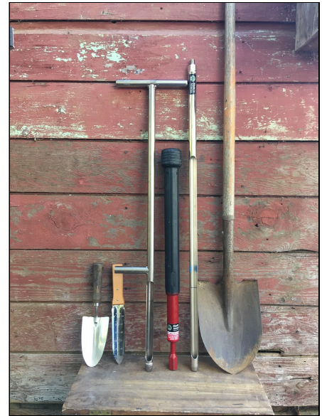
Figure 3. Soil sampling tools, from left: trowel, hori hori knife, probe, hammer probe (in two pieces), and a long-handled shovel.
