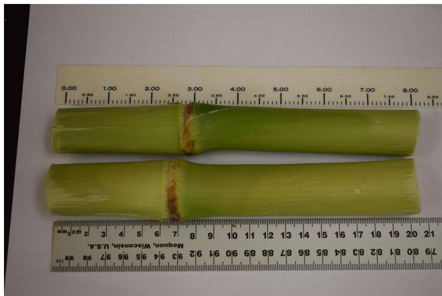
Figure 4. Prepare cornstalk for analysis by removing leaves and leaf sheaths.
