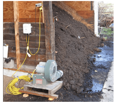
Blowers can be plumbed to push air through the pile, pull air from the pile, or alternate air flow direction.
