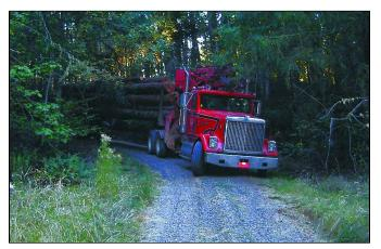
Clearance requirements for personal vehicles are much different than those for logging trucks and logging equipment, especially in terms of turning radius and steepness.
