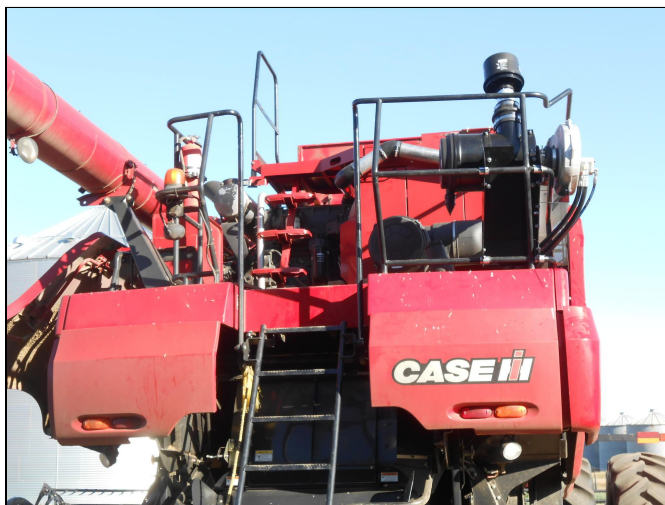
Figure 2. Air intake filter and pressure blower system in the upper right created by DSH Engineering.
