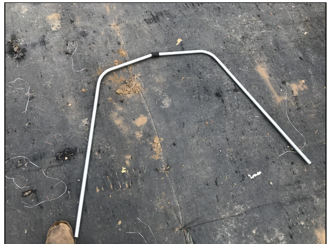
Figure 3. Galvanized electrical conduit is a sturdier option for low tunnel hoops.
