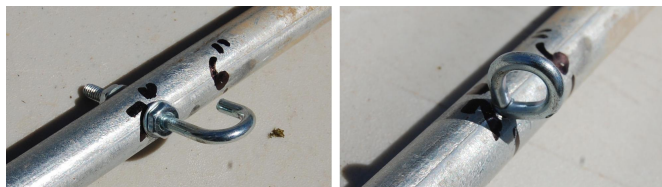
Figure 13. You can use looped bolts or eyehooks as alternatives to the stakes.
