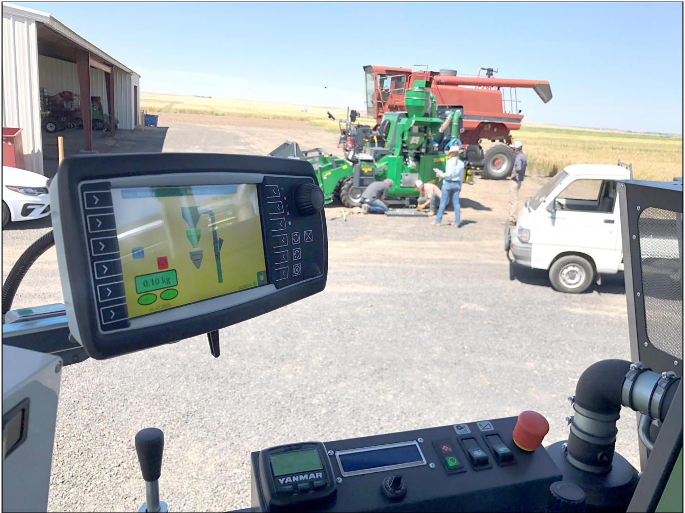
Figure 5. The driver's view of the WieSEL on-combine weight system.
