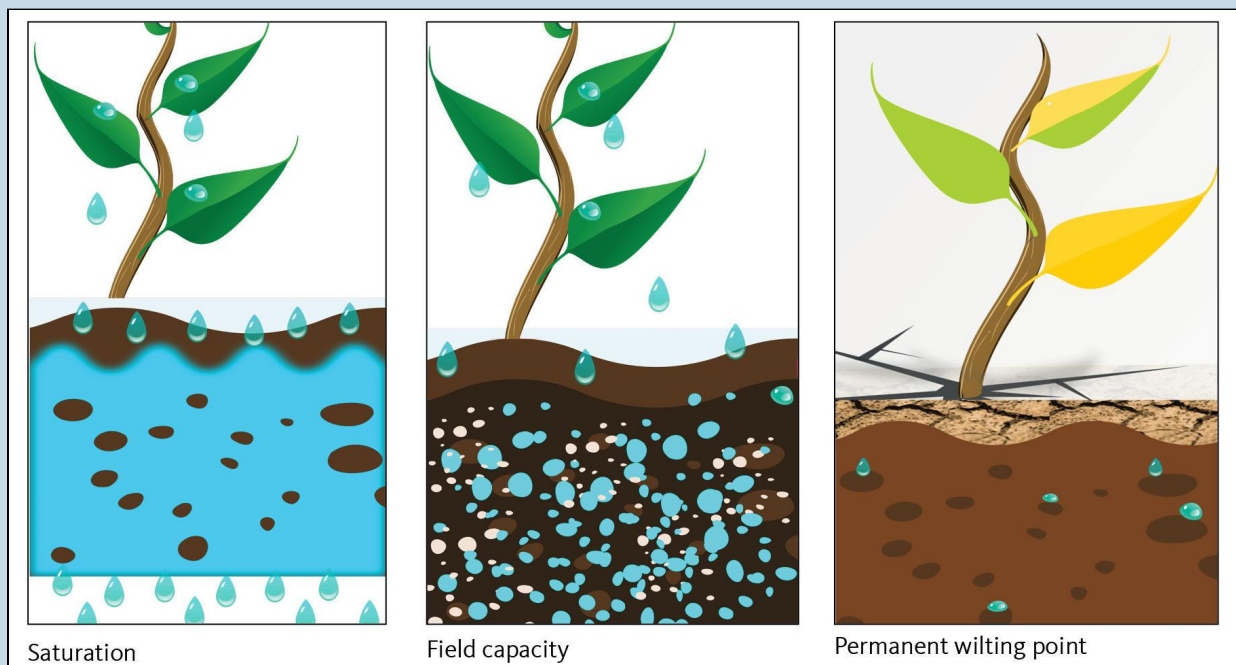
Illustration of saturation, field capacity and permanent wilting point.
