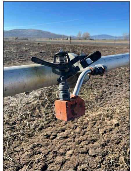
Figure 5. A sprinkler with a leveler (the red part the nozzle is attached to).
