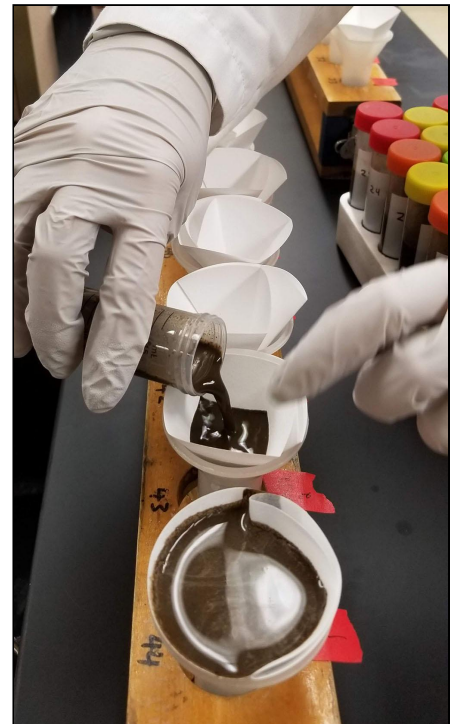
A technician conducts a soil extraction procedure for nitrate and ammonium analysis.
