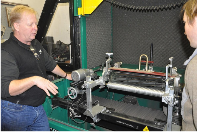
Figure 3. Reels (above) and bed knives (right) require specialized grinding equipment to maintain a high quality of cut.
