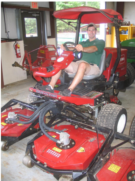
Figure 2. Rotary mowers (above) should be used on turf maintained at heights higher than 1 inch, while reel mowers (right) are best for turf maintained at heights of 1 inch or less.
