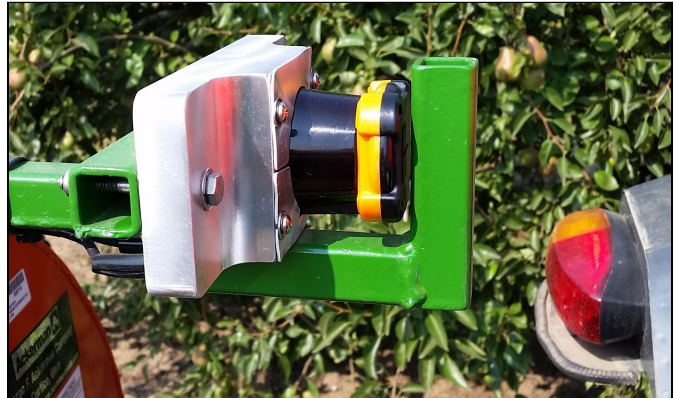
Figure 2B. LiDAR sensor is used in the "Intelligent Spray System" (UTM-30LX/LN Hokuyo Automatic Co. Ltd., Osaka, Japan).
