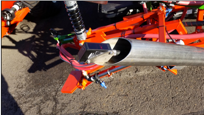
Figure 2A. Infrared sensor used in sensor sprayer applications (QMT42, Banner Engineering, Minneapolis, Minnesota).
