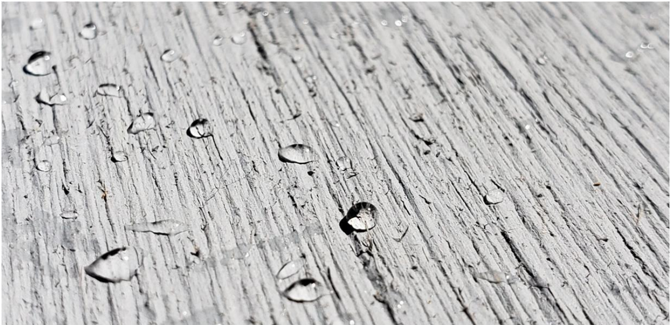
Figure 7. Water beads on the surface of wood treated with a water-repellent wood protection system.
