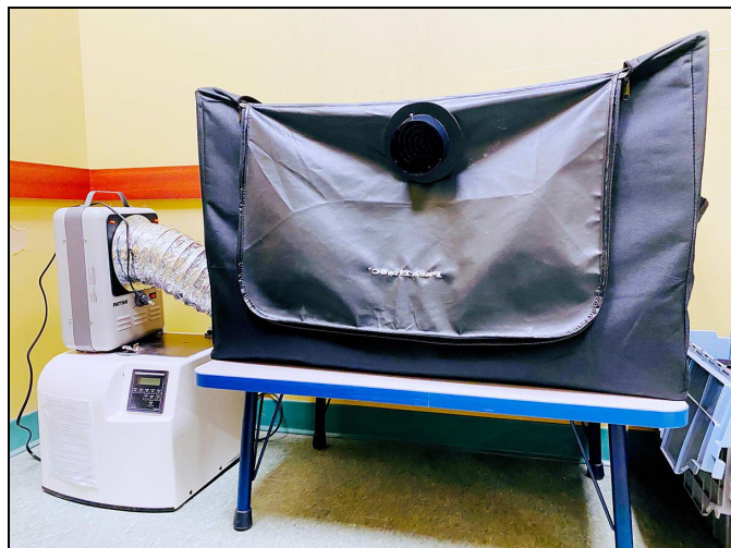
A heat treatment chamber. Densely packing items into heat chambers results in cool spots that bed bugs can survive in. The interior must reach a temperature of 50°C (122°F) for at least four hours to kill all life stages of bed bugs.
