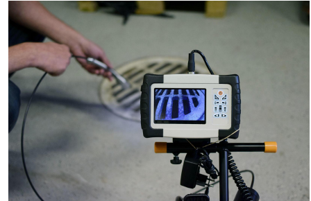
Figure 11. A borescope is a very useful tool for inspecting the insides of drains and plumbing.
