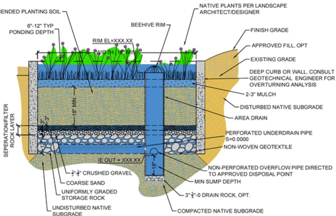
**Figure 2:** Infiltration Stormwater Planter with Planting Soil & Rock Trench
