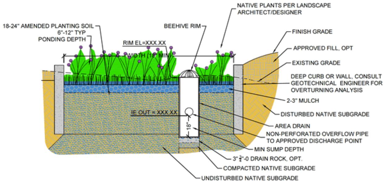
**Figure 1:** Infiltration Stormwater Planter with Planting Soil
