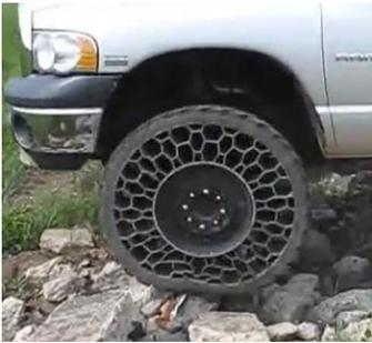
right. Prototypes for honeycomb airless tires are currently in development.
