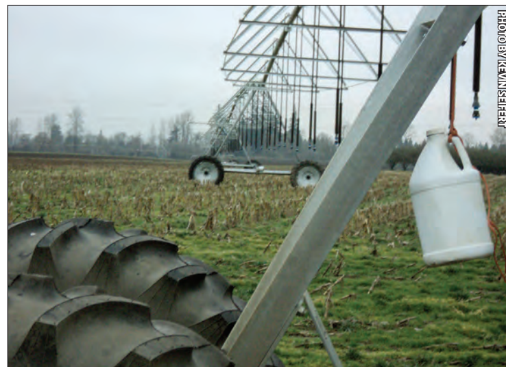
Linear installed in Linn County using LEPA delivery systems.
