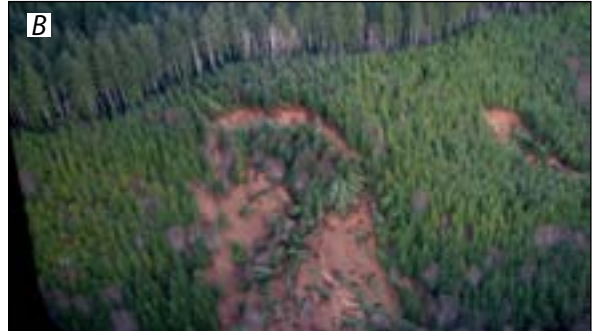
Figure 4.4. A, diagram of a debris avalanche; B, debris avalanche in southwest Washington.
