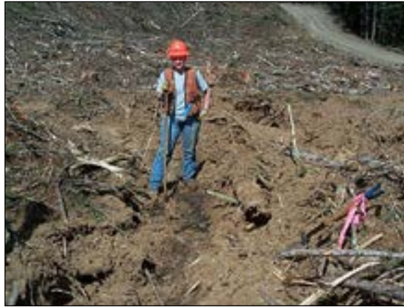
Figure 5.7. Soil disturbance Class 3.
