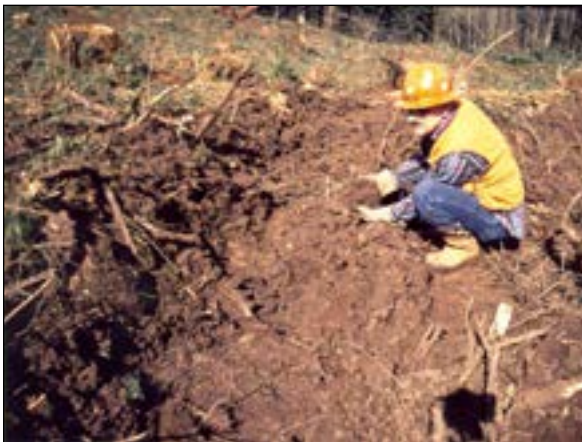
Figure 5.6. Soil disturbance Class 2.
