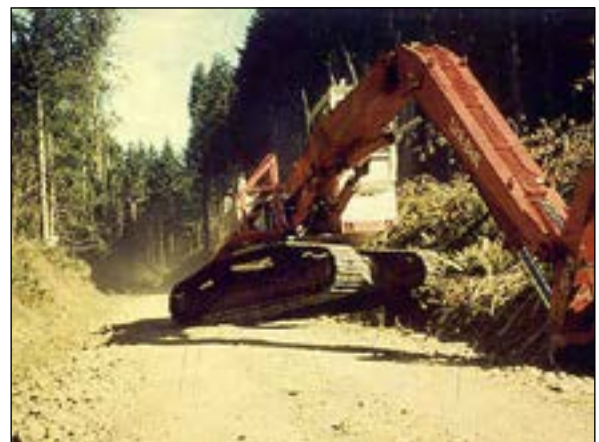
Figure 5.21. Use the shovel's boom to assist turning on the road to enter a setting and to lift up the front of the machine.
