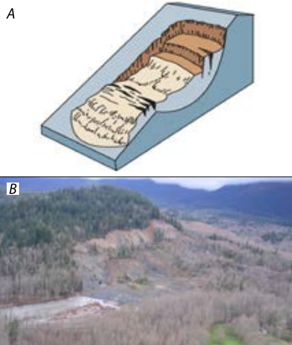
Figure 4.2. A, diagram of a slump-earthflow landslide; B, slump-earthflow along the North Fork Stillaguamish River in Snohomish County, Wash.
