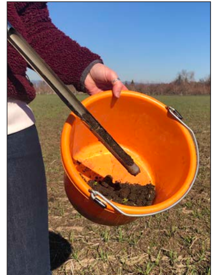
Photo: Gordon B. Jones, © Oregon State University Combine 15–20 soil cores from each management unit to make one composite sample to submit for analysis.
