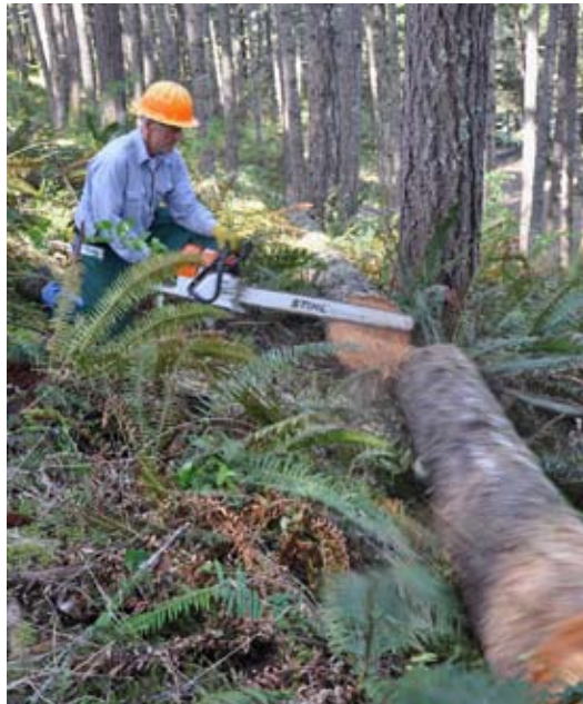
Figure 11.—When bucking, maintain a safe working position on the uphill side of the tree or bucked log. Note that the just-bucked log segment at right is rolling swiftly downhill.
