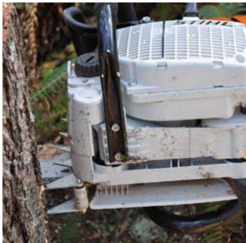
Figure 7.—Saw dogs, the sharp teeth on the left side of this saw, greatly improve your safety and cutting accuracy.
