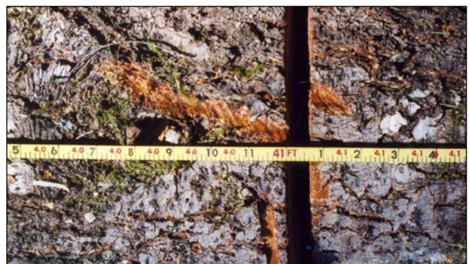
Figure 3. A combination logger's tape (above) can measure tree diameter in addition to log lengths (below).
