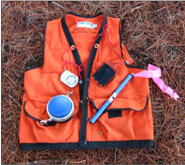
Figure 1. Tools you'll use for some measuring tasks are (clockwise, from top left) a clinometer, a compass, an increment borer (with flagging tape attached to make the borer easier to find if it falls on the ground), and a combination logger's tape.
