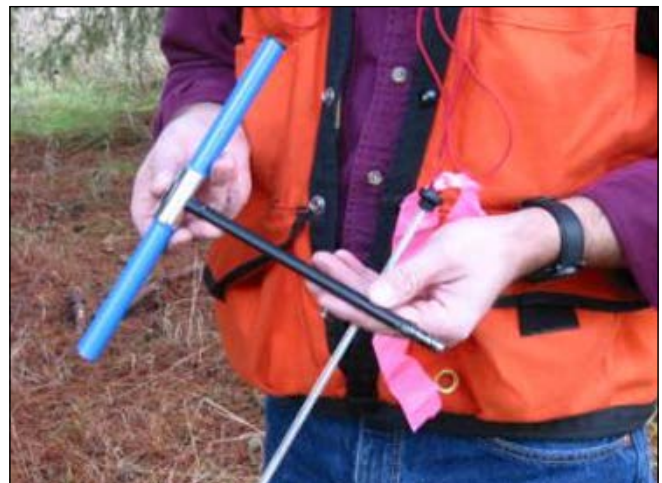
Figure 6. A core sample obtained from a tree with the increment borer allows you to determine a tree's growth rate.
