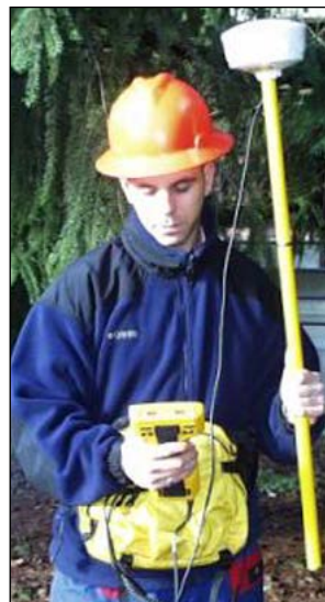
Figure 5. Consumer-grade GPS units are less expensive and less accurate than mapping-grade GPS receivers, but they help make rough length or area measurements.
