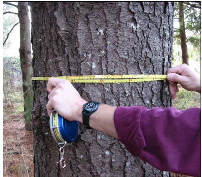
Figure 3. A combination logger's tape (above) can measure tree diameter in addition to log lengths (below).
