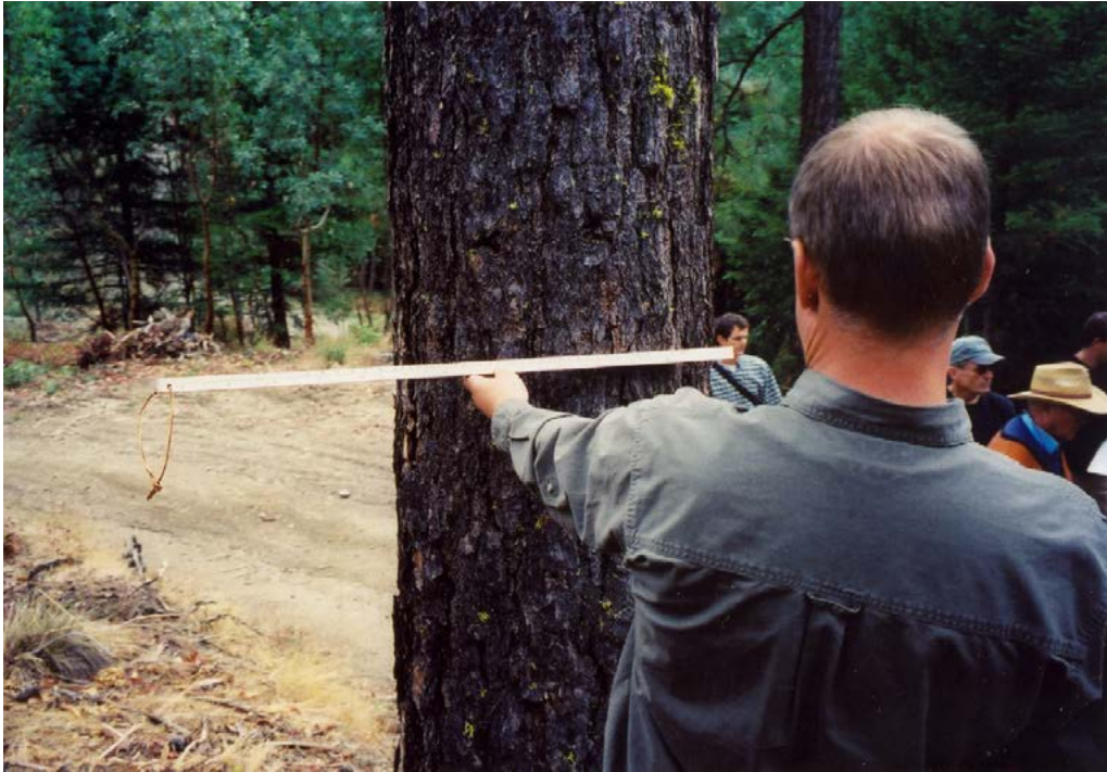
Figure 8. The Woodland Stick is an easy-to-use and moderately accurate tool for measuring tree height and diameter. It must be held 25 inches from the eye; at any other distance, it gives incorrect readings.
