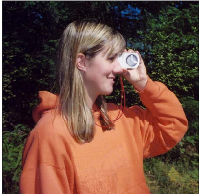
Figure 2. The clinometer has a sighting hole and a suspended circular scale that can measure ground slope as well as tree height.
