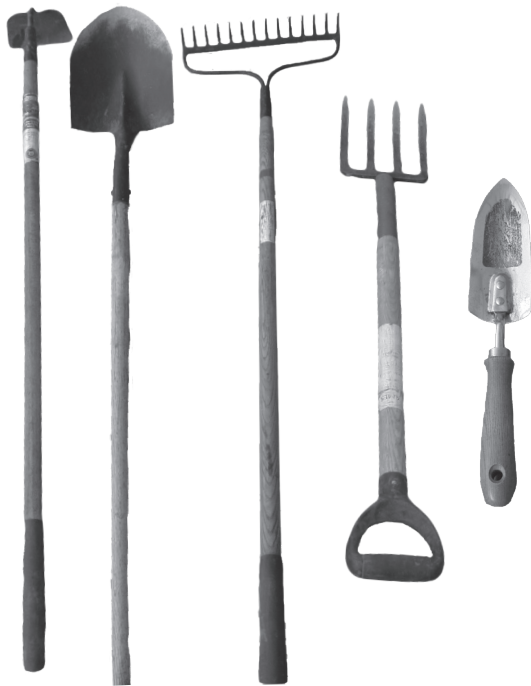
Figure 3. Most gardeners make regular use of ( left to right ) a hoe, shovel, rake, spading fork, and trowel. These tools are available in adult and child sizes (not shown).
