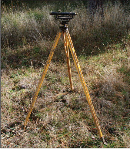
A tripod and level are needed to determine slope when installing culverts or road grades.
