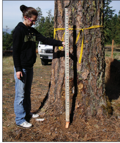
A level stick is used in conjunction with the level to determine slope.
