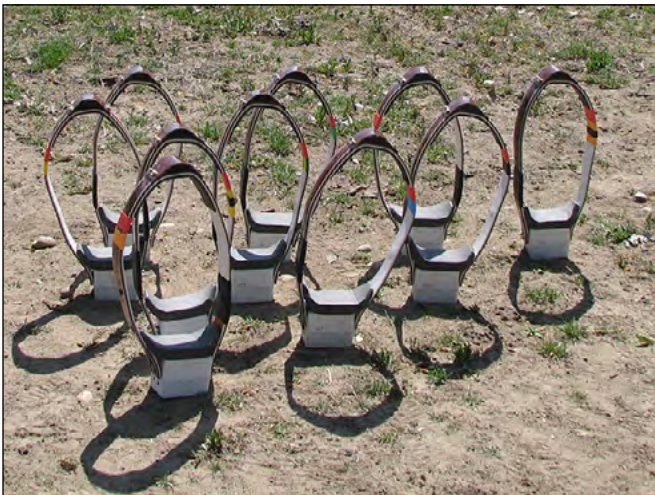
Figure 2. Collars being prepared to place on cattle at one of the research ranches. Animal tracking collars used in the project were developed over the last 10 years by Dr. Pat Clark and Dr. Douglas Johnson, along with cooperating engineers.
