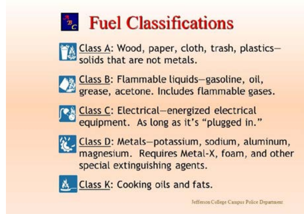
Figure 4: Characteristics Class A,B,C,D and K fuel types.
