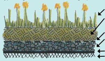
Plants Sedums, grasses, shrubs, trees Growing medium 4–36 inches, depending on plant choice **Filter fabric** Alternatively, substitute 3 inches of coarse sand over 3 inches of crushed rock (3/8-1/2 inch)**Drainage layer** Optional with well-drained growing medium. Materials may include rocks or manufactured drainage mats. Waterproofing Roof/structural support
