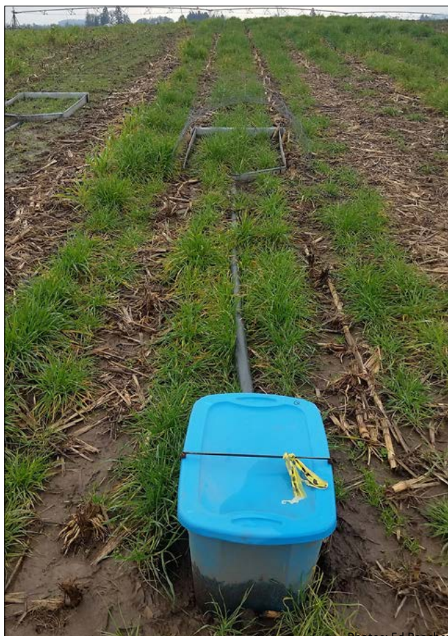
Figure 10. Microplots were used to estimate the effect of cover crop establishment method on soil erosion.
