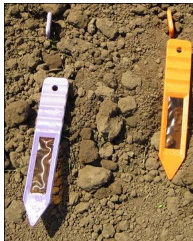
Figure 8. Plant Root Simulator probes. In our experiments, probes were inserted vertically into the soil between corn rows, on zero P (no fertilizer) plots. PRS probes adsorb cations (left, purple) and anions (right, orange) from soil solution, using a charged resin sheet. When inserted into soil, the window of PRS probes (with exchange resin) was at a soil depth of 3–5 inches.
