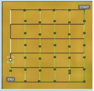
Figure 6. Screenshot of a unmanned aerial system flight in progress using a double-grid flight plan to ensure adequate image collection. The unmanned aerial system location is indicated by the red and green quadcopter icon. The green line indicates flight path already traveled, in this case, it has almost completed the white-lined part of the double-grid pattern and will next fly the black-lined pattern. The camera icons show locations of each image capture along the route.
