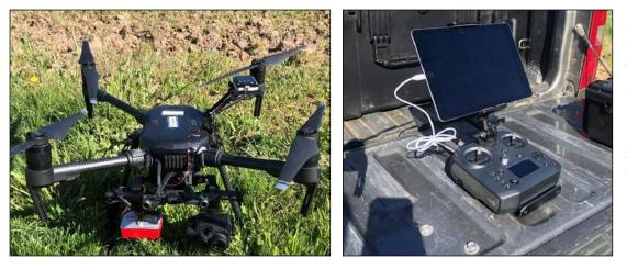
Figure 3. An example of a quadcopter (left) and a controller with a tablet attached to aid in flight path planning and image capture (right). A mast holds a GPS and light sensor above the rotors. The payload is a dual camera gimbal with a multispectral camera and an IR/ RGB camera.
