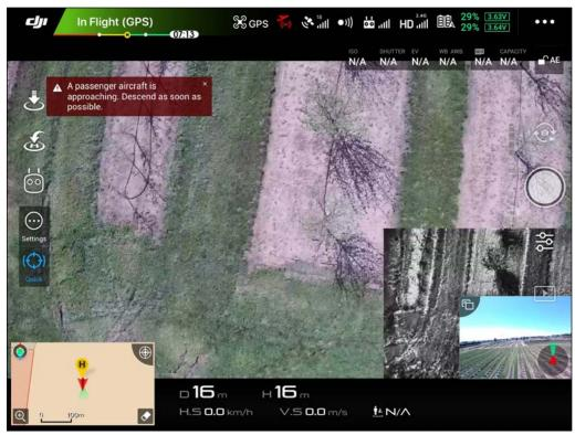
Figure 4. Screenshot of a flight display on a tablet during an unmanned aerial system flight. The display includes many inputs, including the RGB image (large image), the IR image from the same camera (lower right), and the flight path camera (smallest image lower right). Other information displayed includes battery remaining (upper right), GPS status (upper middle), flight path confliction (upper-middle and upper left warnings, controlled airspace shown lower left).
