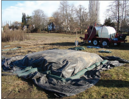
Photo: Marianne Elliott, Washington State University Figure 35. Sanitizing soil with steam.
