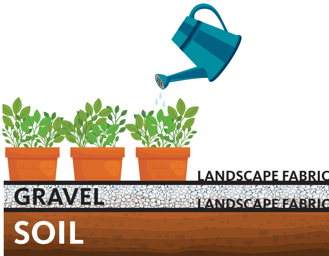
Figure 27. A “gravel sandwich” is created by placing landscape fabric below and above a layer of gravel to create a barrier between soil and plants.
