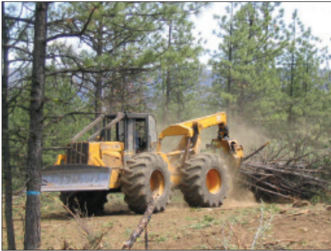
Figure 10.5. Rubber-tired skidders can skid logs at longer distances quickly, work on slopes up to 35%, and are one of the most common skidding methods in eastern Oregon.
