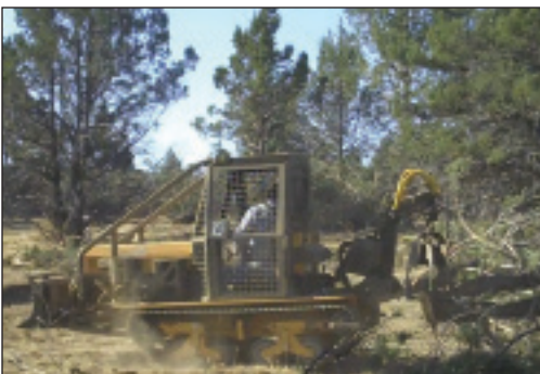
Figure 10.4. Small-scale skidding machines like this one are a cost-effective and low-impact alternative for owners of small woodlands.
