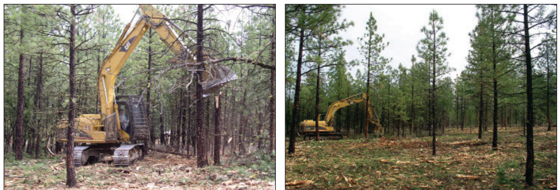
Figure 11.11a-b: A slashbuster thinning and fuel reduction operation is underway in young pine stand. Material is left on ground to decompose.
