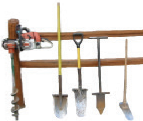
Figure 6.2. Planting tools include the power auger (at left), various types of shovels, and the hoedad (at right).
