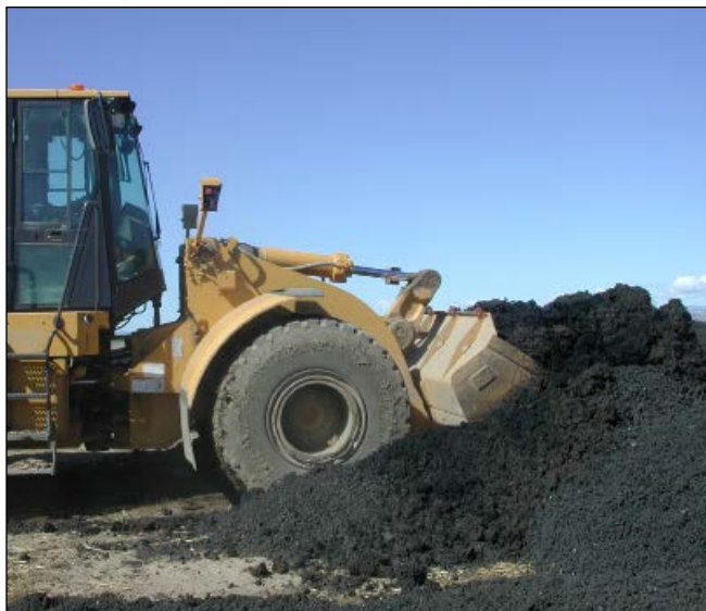
Photo: Andy Bary, ©Washington State University Dewatered biosolids stockpile at field application site
