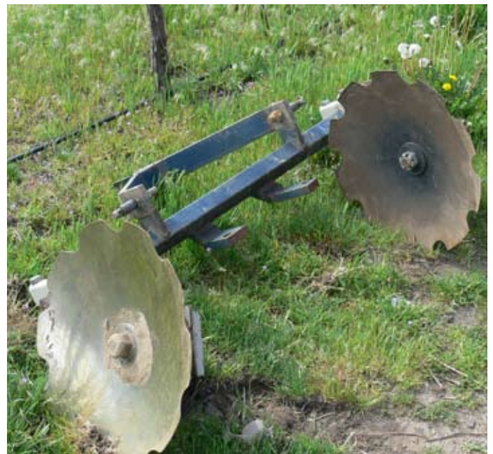
Figure 9. Plough with angled blades for cutting a 4-inch V-trench.
