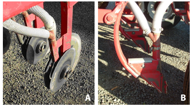
Figure 3. The customized Fabro drill places fertilizer below and beside the seed using double disc blades (A). Double disc blades are mounted on a separate gang in front of narrow, hoe-type (atom jet) seed openers (B) on 12-inch row spacing.
