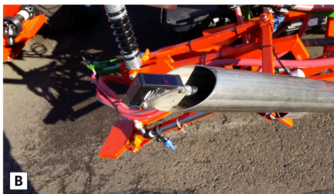
Figure 2: (A) Infrared sensor used in sensor sprayer applications (QMT42, Banner Engineering, Minneapolis, Minnesota; (B) LiDAR sensor (UTM-30LX/LN Hokuyo Automatic Co. Ltd., Osaka, Japan) used in the “Intelligent Spray System”.
