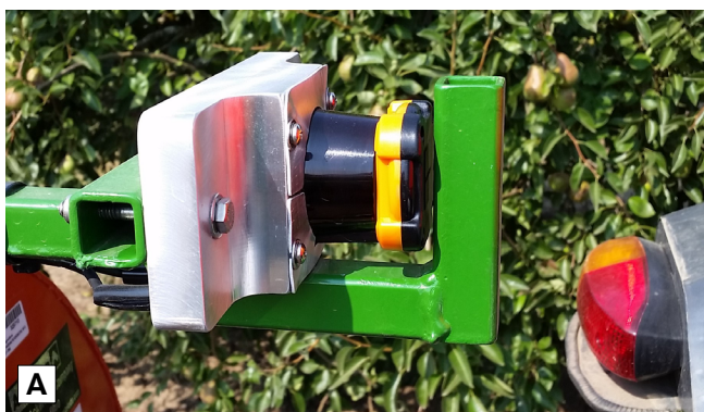
Figure 2: (A) Infrared sensor used in sensor sprayer applications (QMT42, Banner Engineering, Minneapolis, Minnesota; (B) LiDAR sensor (UTM-30LX/LN Hokuyo Automatic Co. Ltd., Osaka, Japan) used in the “Intelligent Spray System”.
