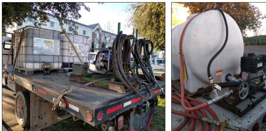
Figure 2: A truck deck (left) with pump and hose secured on pallet and two IBC totes that serve as feed tanks. At right is a close-up of a feed tank, pump and hose setup on a truck bed.
