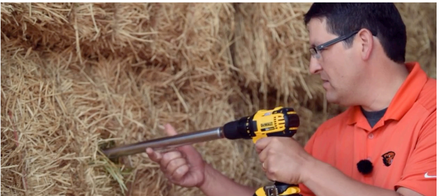
A hay corer is the best way to collect a sample for laboratory testing. Credit: Oregon State University
