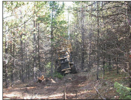
Figure 8. An all-surface vehicle with Slashbuster head thins a young western larch stand.
