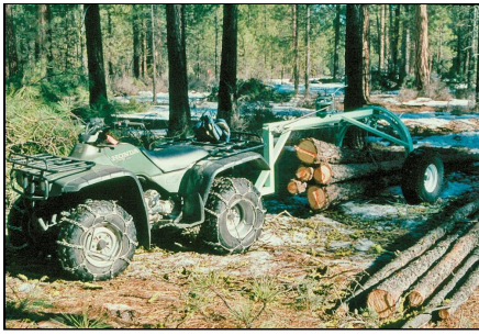
Figure 7. This ATV with a “log arch” is an example of light-duty harvesting equipment for small-diameter logs.
