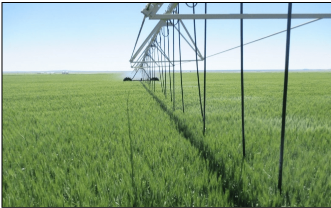
Figure 7. A low-elevation spray application operating in a wheat field with the sprinkler heads below the top of the canopy.
