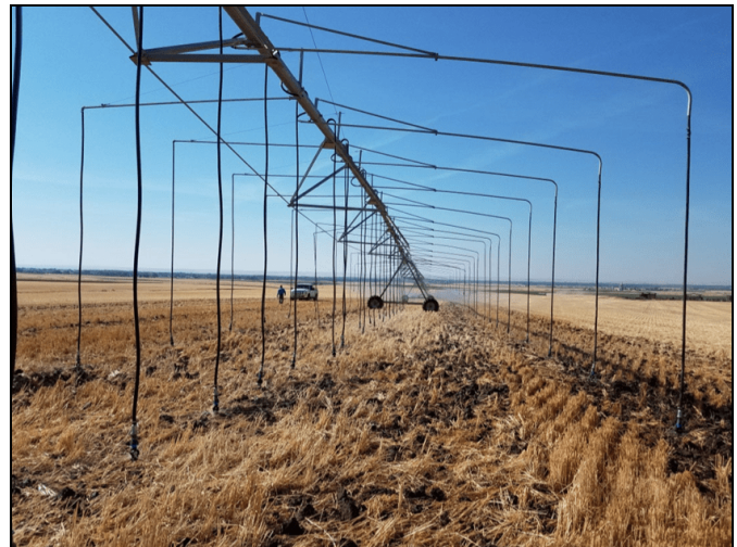
Figure 8. This low-elevation spray application system uses boombacks to spread the water out and increase infiltration on a wheat field near Milton-Freewater, Oregon.
