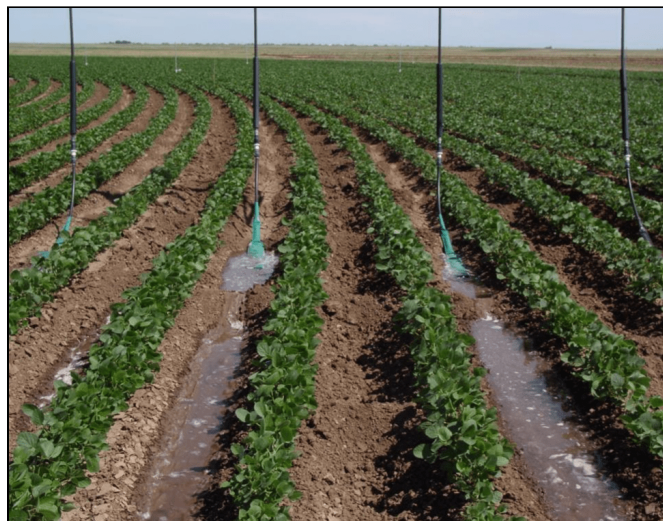
Figure 10. A low-energy precision application system on a row crop using drag socks to minimize erosion to the furrow dikes that limit water movement in the furrows.
