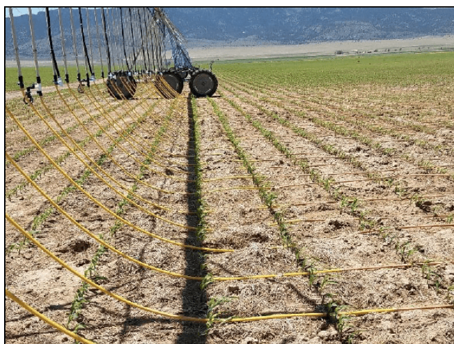
Figure 11. Mobile drip irrigation system installed on a center pivot with drip lines attached to rigid drop tubes and placed along crop rows to apply water directly to the soil surface.
