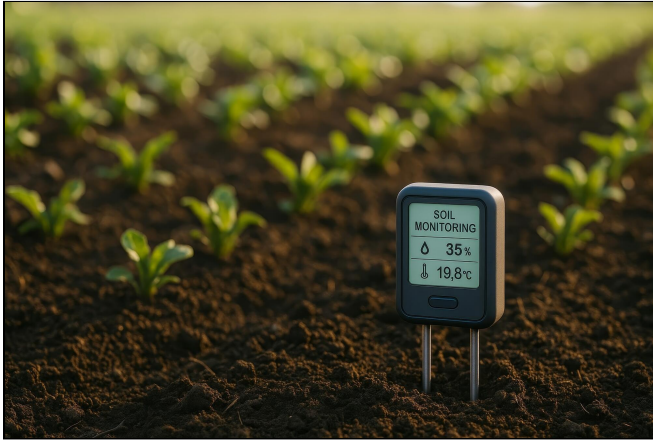
Figure 7A. A time-domain reflectometry (TDR) soil moisture probe measuring real-time soil moisture in the field.
