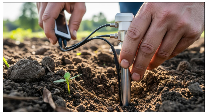
Figure 10. Proper installation of a soil moisture sensor within the crop root zone. Sensors should be installed in representative management zones with firm soil contact and minimal disturbance to ensure accurate, reliable readings for irrigation decision-making.
