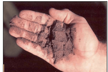
Figure 3. Determining soil moisture using the feel and appearance method.
