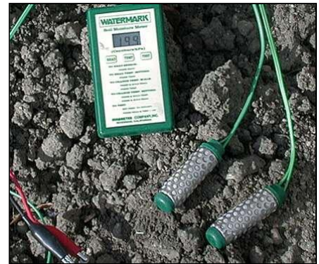
Figure 6. Watermark granular matrix sensors connected to a handheld data analyzer used to measure soil water tension in the field. Sensor readings can be used to monitor root-zone moisture conditions and assist with irrigation scheduling.
