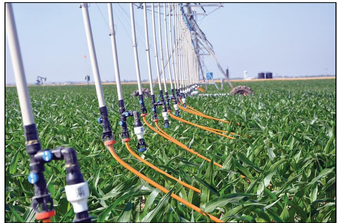
Figure 15. Mobile drip irrigation installed on a center pivot system. Water is delivered through drop hoses connected to drip tubing placed on the soil surface, allowing irrigation water to be applied directly to the root zone.
