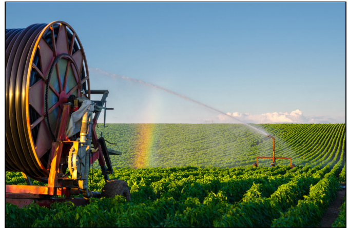
Figure 11B. A traveling gun applies irrigation water as the hose reel slowly retracts and pulls the sprinkler cart across the field.
