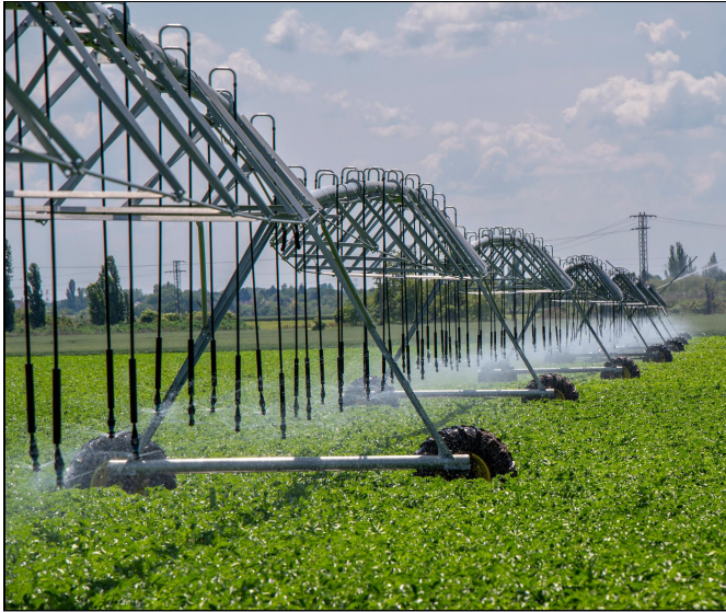
Figures 13A. A low-elevation spray application package on a lateral-move irrigation system.
