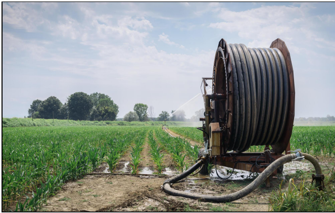
Figure 11A. A hose-reel irrigation machine with a flexible hose supplies water to the traveling sprinkler cart.
