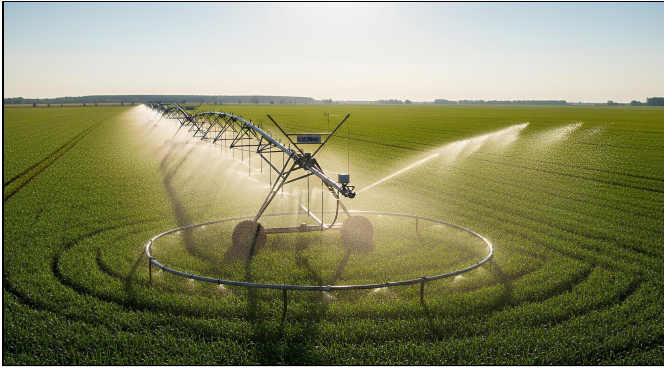
Figure 12A. A center pivot irrigation system used for large-scale field irrigation. These systems apply water uniformly while moving across the field.
