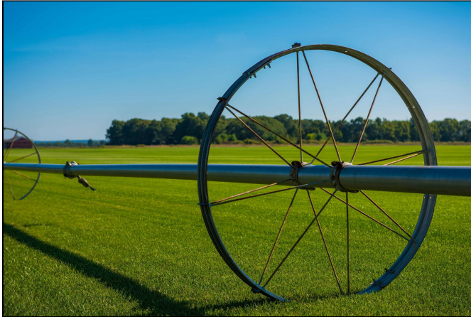
Figure 7A. A wheel line (side-roll) irrigation system used for field crop irrigation. The wheel and pipeline structure allows the system to roll across the field between irrigation sets.
