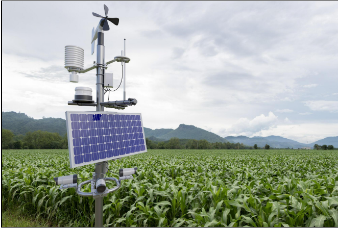
Figure 6. Weather station data are used to estimate reference evapotranspiration, or ET_0 , a key input for irrigation scheduling. Combining climate data with crop information helps determine crop water requirements and improve irrigation efficiency.
