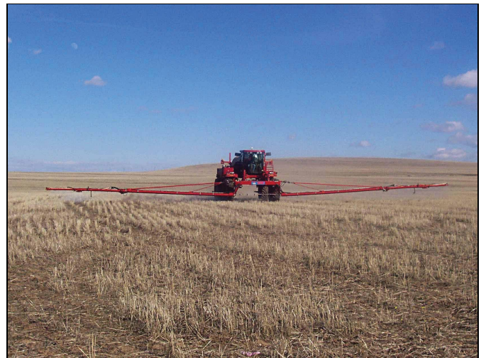
Figure 2. Weed control applications in commercial-sized fields are often made with large, self-propelled sprayers capable of treating 800 acres or more in a single day.
